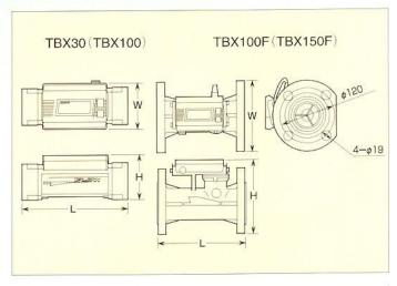
The display unit on the TBX100F (TBX150F) can be freely moved about to match the gas flow direction. In addition, the entire display unit can be removed and placed up to three meters away.
